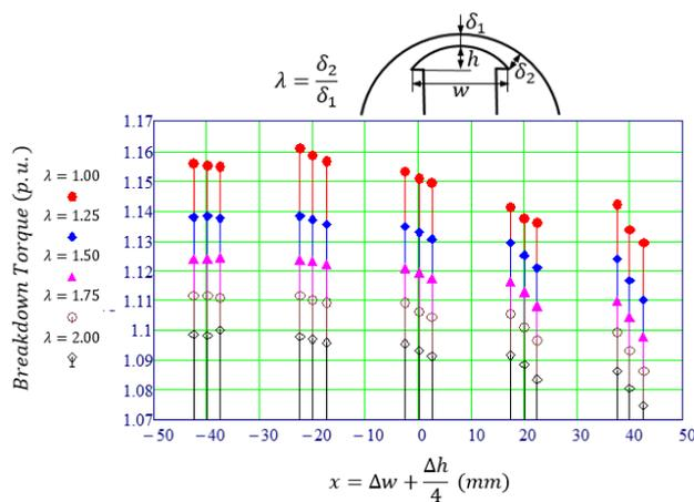
Figure 6: The variables of the parametric study, which determine the pole shoe geometry, are shown on the top of the picture. The obtained results in the form of the breakdown torque are presented. The width (5 steps) and height (3 steps) of the pole shoe was changed with a step of 20mm and of 10mm respectively. The height difference is divided by 4 so that the changes of the height for each change of the width produce a group with three designs.
