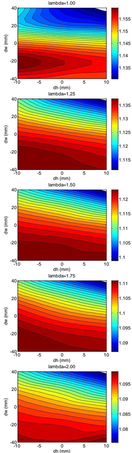
Figure 7: The breakdown torque of the chosen motor as a result of the parametric study defined in Figure 5 is depicted.
