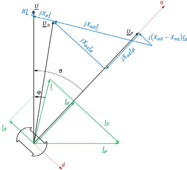
Figure 1: The vector diagram of the considered ABB synchronous motor with salient pole rotor (15.6MW, 3'900V, 5.6Hz) at the nominal operating point is presented.
