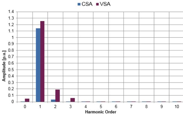
Figure 5: The Fourier analysis of the torque curves presented in Figure 4. The fundamental frequency of this analysis is 5.6Hz (the harmonic order 1).
