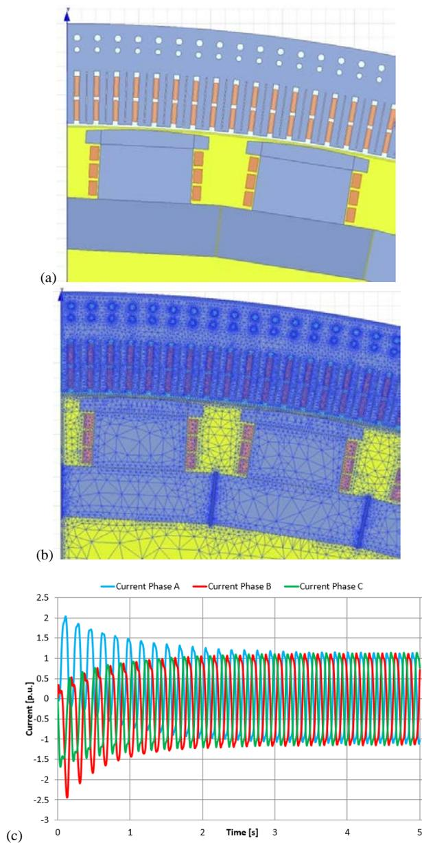
Figure 2: The geometry (a), FEM mesh (b) and the motor’s currents over the transient solution process (c) by using the described VSA. A typical ABB synchronous motor with salient pole rotor (15.6MW, 3’900V, 5.6Hz) is considered.
